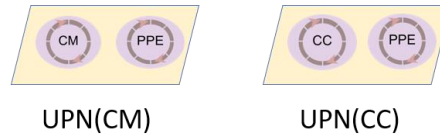
Figure 3. UPN(CM): UPN of a micro cell managed by a CM, and UPN(CC): UPN of a macro cell managed by the CC.
