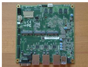
Figure 29. 5GNaaS SDN hardware switch board.
